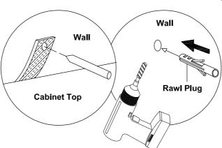
Drill a hole in the wall and insert the rawl plug.
