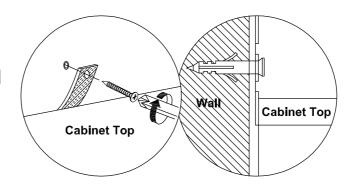
NOTE: Wall fixings are not supplied with this product as different wall materials require different types of fixing devices (such as Rawl plugs on brick work). You must use fixing devices suitable for the type of wall you intend to mount this product to.Please ensure that the head of any screw used as a diameter greater than the diameter of the mounting hole on the bracket and that the fixing is safe and secure before use.
