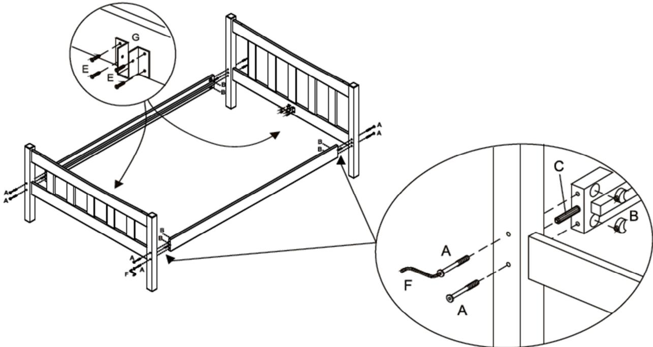
Step 2: Fix the centre rail (5) into hardware part G using hardware part E and a screwdriver (not provided). DO NOT use any power tools as this may damage the frame and will invalidate any claim.
