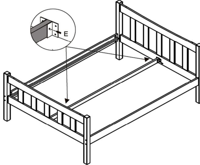
Step 3: Fix the slats (4) to the side rails (3) working from the ends to the middle, using hardware parts D and H with a screwdriver (not provided).
