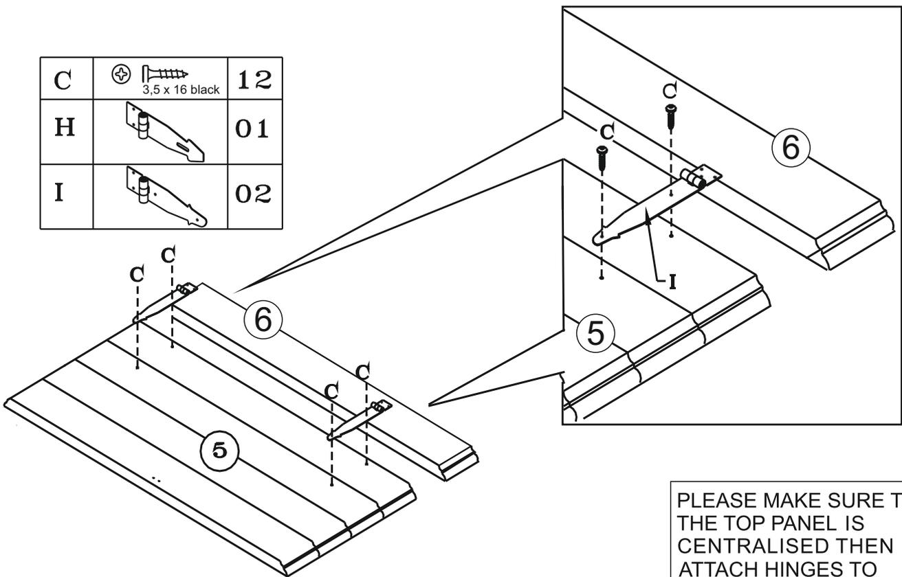
PLEASE MAKE SURE THAT THE TOP PANEL IS CENTRALISED THEN ATTACH HINGES TO PART 6 USING SCREW C.
