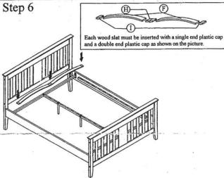
Once both wood slats have been inserted with the plastic caps, fix it on the wood side rails and center bar by pressing it accordingly to the default holes. Ensure the plastic cap's pin is aimed to the hole. At last make sure all screws and bolts are tighten.
