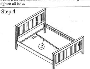
Fix center bar 'D' to cross bar 'E' by follow like diagram as shown.
