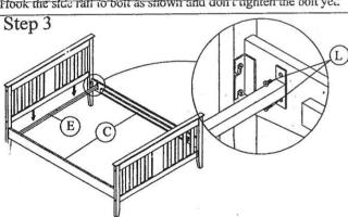
Put in cross bars and fix in bolt 'L' as shown in diagram and tighten ali bolts.
