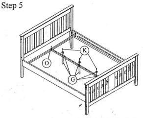
Fix center bar with bolt 'O' and tighten it. After that fix in support leg with bolt 'K'.
