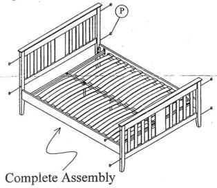
Make sure all bolts are tighten. At last insert wood button (P) as shown.
