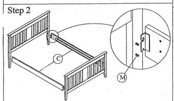
Flook the side rall to bolt as shown and don't tighten the bolt yet.
