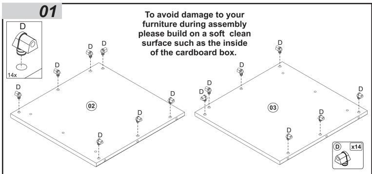
Insert part (D) into the marked hole by pushing and turning clockwise at the same time until fully inserted and flush with the surface, or push part (D) into holes and gently hammer until flush with surface and facing forward.
