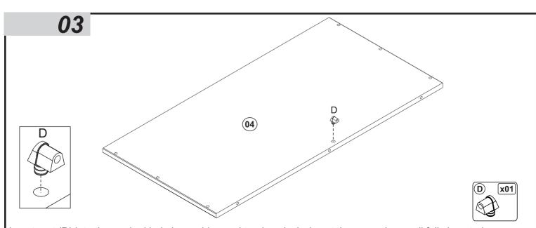
Insert part (D) into the marked hole by pushing and turning clockwise at the same time until fully inserted and flush with the surface, or push part (D) into holes and gently hammer until flush with surface and facing forward.
