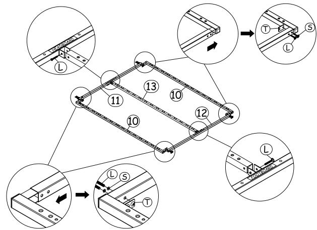
**Step 7**: Attach hardware parts **J** and **K** using hardware part **L**. **Important note: Please assemble follow arrow direction.**
