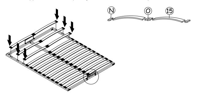
**Step 9**: Assemble the bed base on the right & left hydraulic frame and fix bolts  $\bf M$  starting from ' 10.1 ' to ' 10.3 ' as shown and stick it the self adhesive  $\bf U$  as shown.
