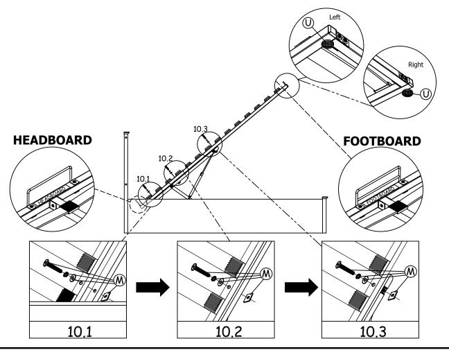
**Step 10:** Assemble the support leg (14) to the bed base as shown. Important note: **Do not tighten the bolts yet!, and this assemble must be done by two persons.**
