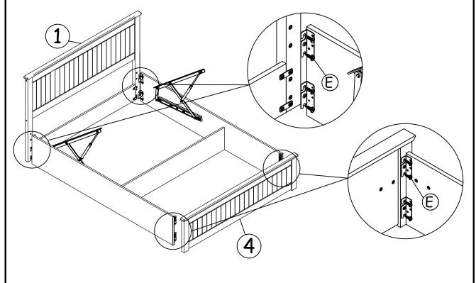
**Step 5**: Fix metal corner block  $\bf C$  to the edge of footboard and side rails with bolt  $\bf F$  as shown. DO NOT use any power tools as this may damage the frame and will invalidate any claim.
