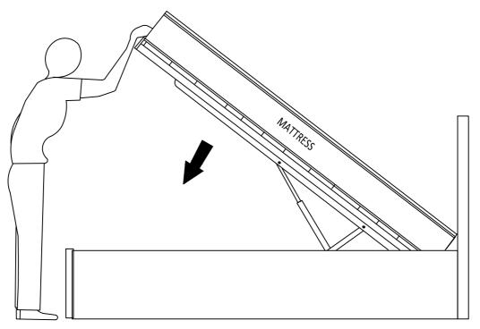
WARNING: Take care when assembling the base. Assemble the ottoman as closed to its final position. The Ottoman has a powerful, mechanism and after assembly should only be opened when the mattress is in place.
