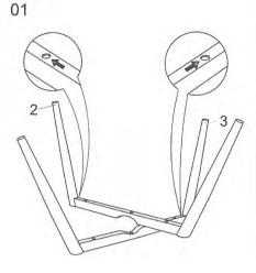
Slot legs together ensuring the arrows on the legs are facing the correct way.
