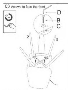
ARROWS TO FACE THE FRONT OF SEAT Place the chair legs onto the upturned seat and loose fix
