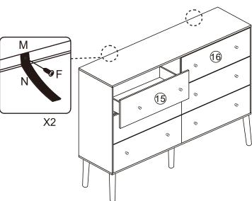
PLEASE NOTE that wall fixings are not supplied as different wall materials require different fixing devices. You must use fixings devices suitable for the type of wall you intend to mount product to. Ensure the head of any screw used has a diameter greater than the mounting hole and the fixing is safe and secure before use.
