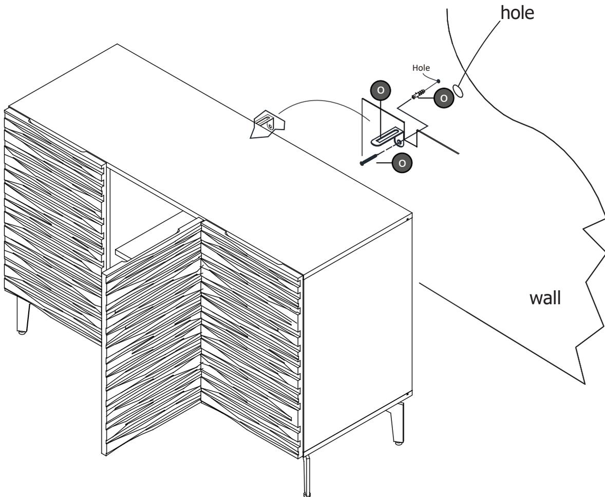
**NOTE :** The wall fixing plug supplied with this product is suitable for solid and brick walls .
