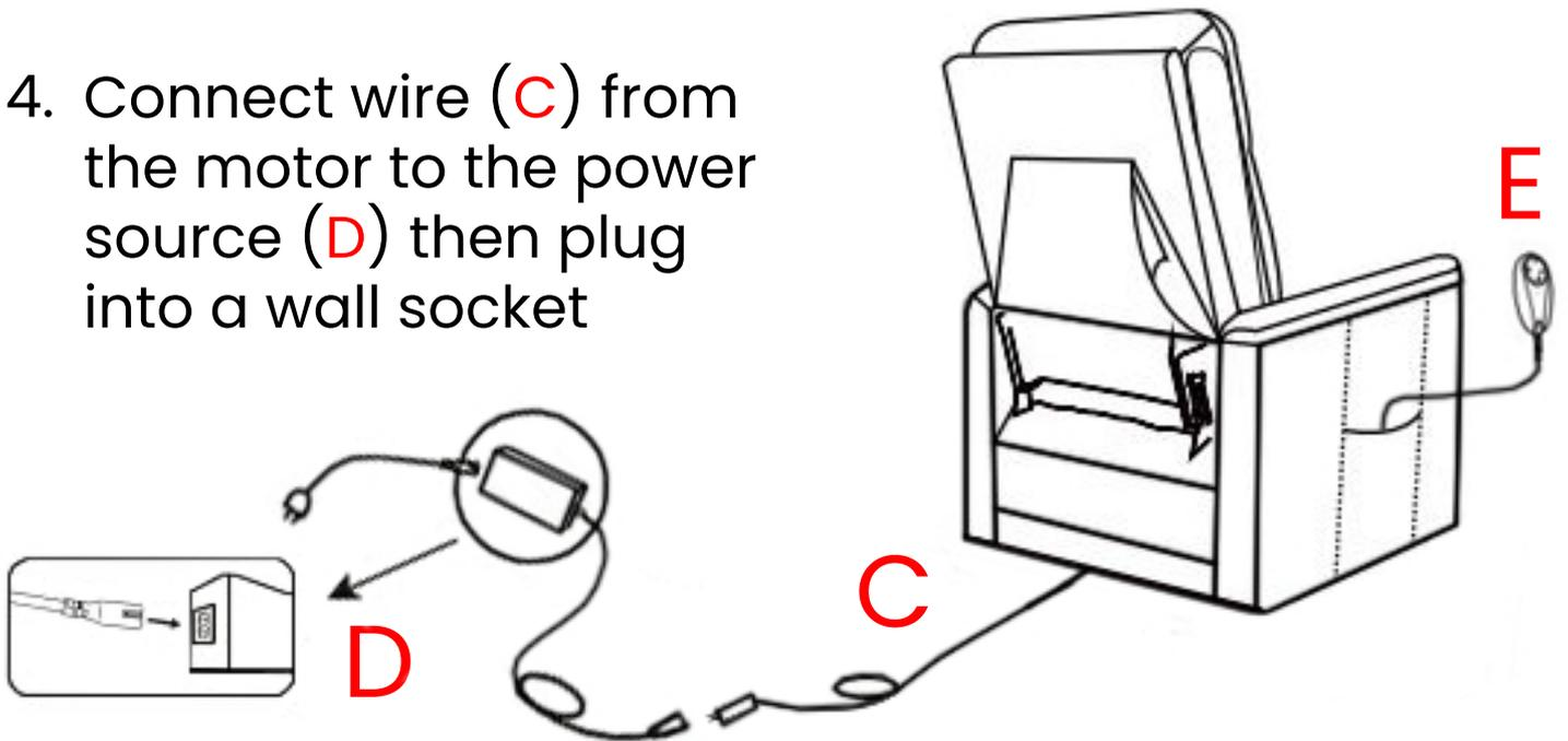
5. Handset (E) is located in the side pocket and is already connected to the mechanism
