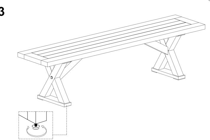
Please adjust levellers in the bottom of the legs if the product does not sit flat on various surfaces
