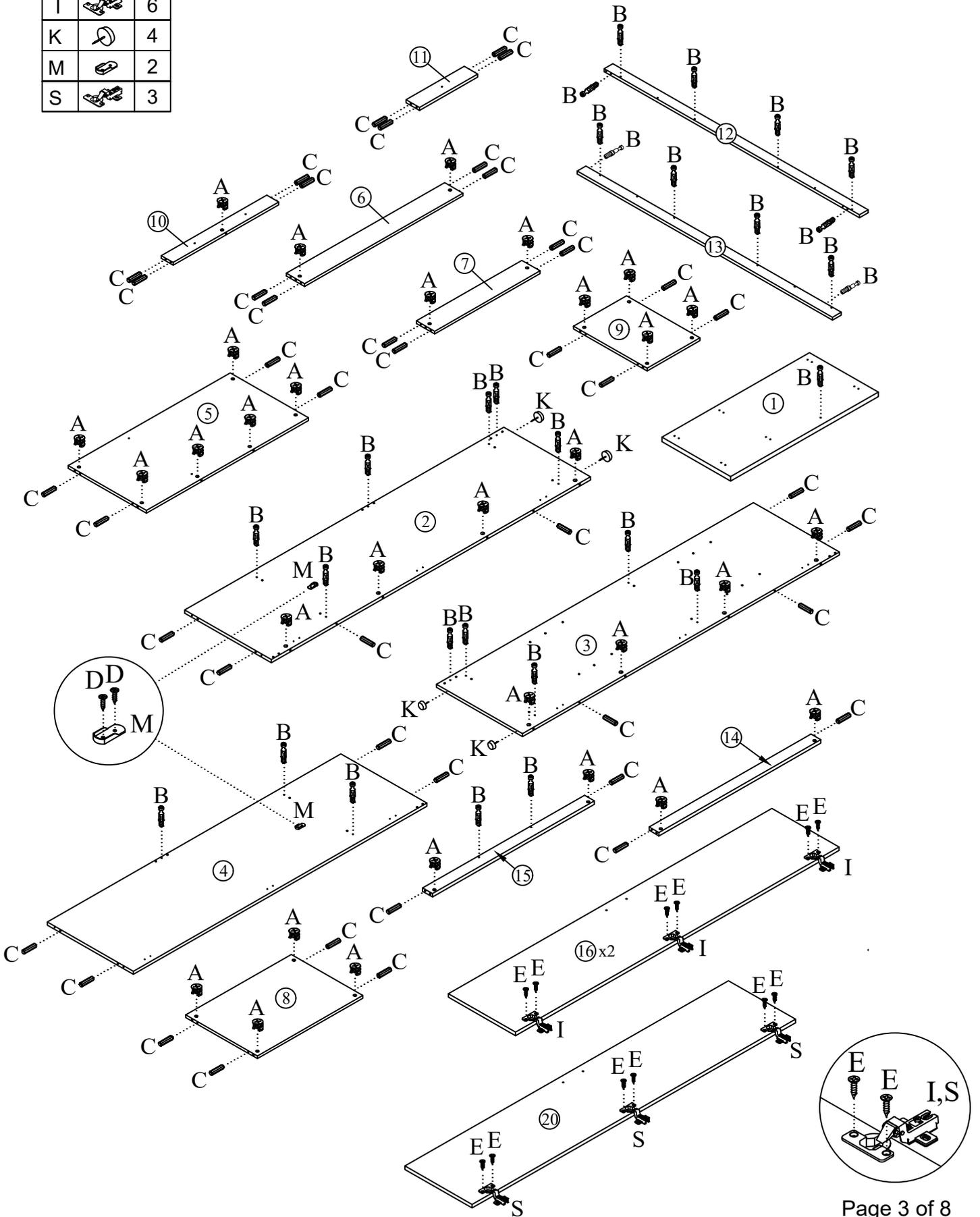
**2** Attach the Post Panel together (12),(13),(14)&(15) by screwdriver (not provided).
