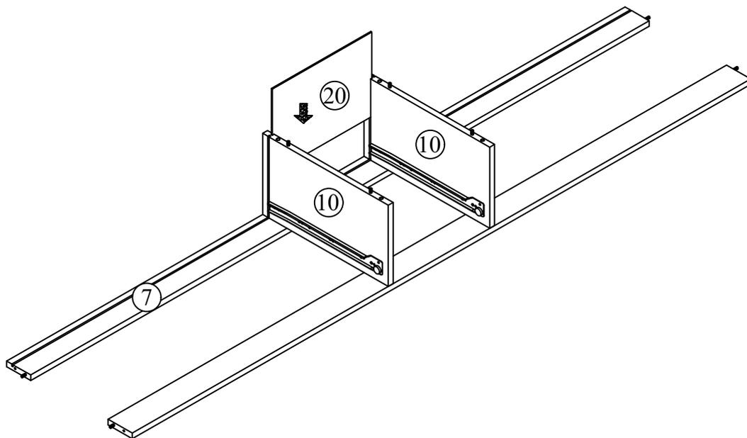
**12** Fix the vertical panel (6) to the center panels (10) by using a screwdriver (not provided). **DO NOT** use any power tools as this may damage the frame and will invalidate any claim.
