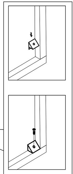
**Step 9:** Secure the safety strap (M) to the back of the table with the washer (L) and screw (F)
