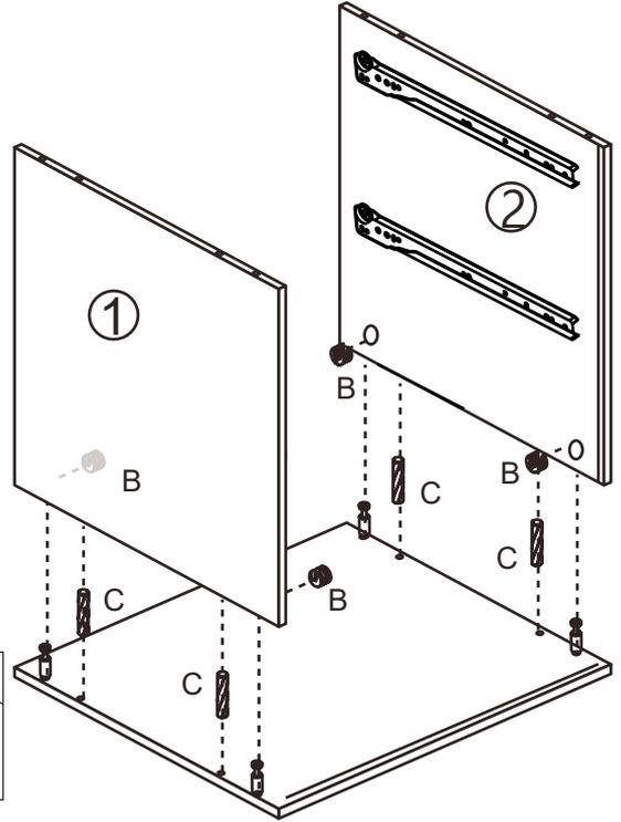
**Step 6:** Slide the back panel (6) into the groove in the side and top panels Push dowels (C) into the bottom of the side panels (1) and (2); then attach the bottom panel (5) using threaded bolts (N)
