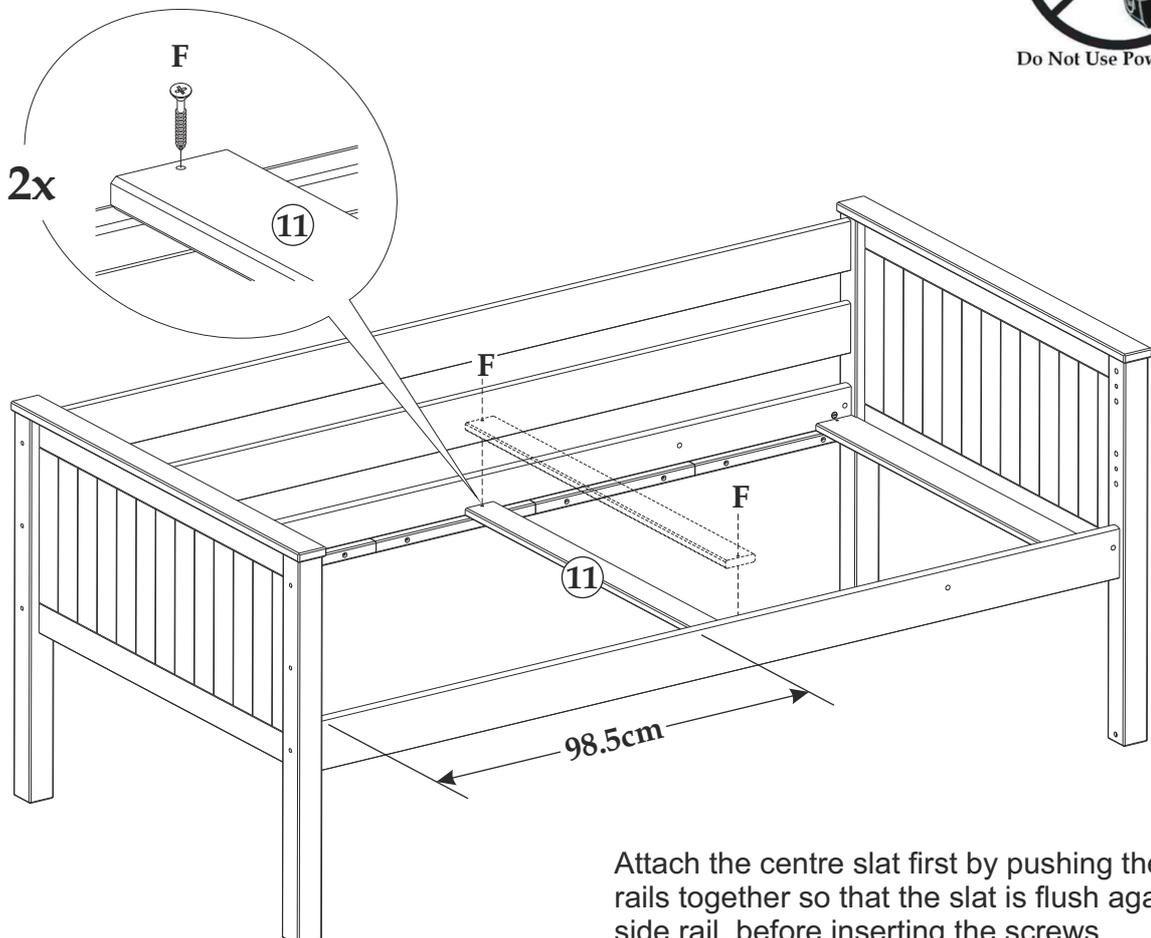
Attach the centre slat first by pushing the side rails together so that the slat is flush against the side rail, before inserting the screws.
