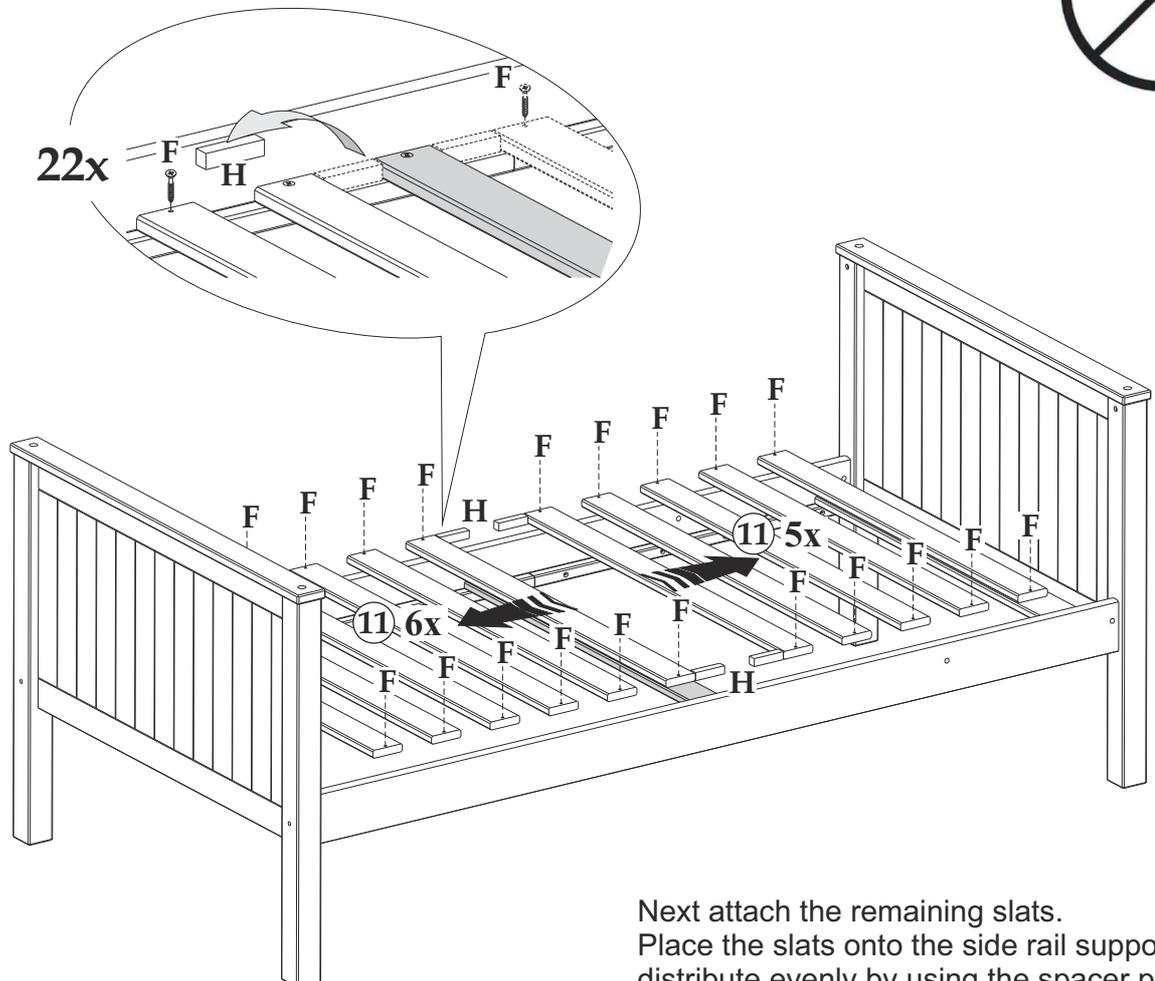
Next attach the remaining slats. Place the slats onto the side rail supports and distribute evenly by using the spacer provided.
