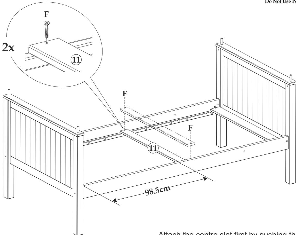
Attach the centre slat first by pushing the side rails together so that the slat is flush against the side rail, before inserting the screws.
