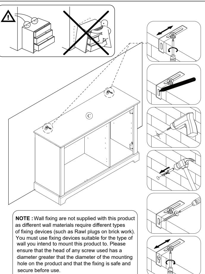
The brackets and screws which to fix the strap
