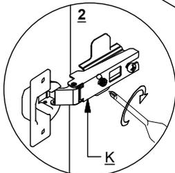
2. LATERAL ADJUSTMENT BY SCREW ADJUSTING
