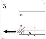
• Ensure the roller is in the track of drawer slide before push to the end.
