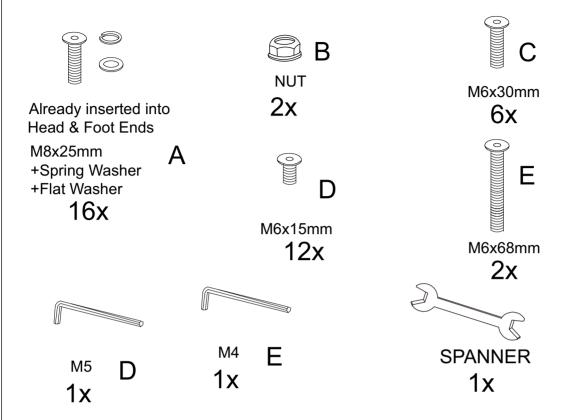
We strongly advise that you do not use Power Tools, such as drills or electric screwdrivers during the assembly as this may cause irreparable damage and will invalidate your warranty.
