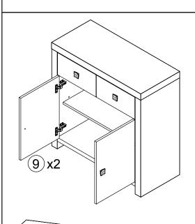
Initially in each door fix 4 screws (E) through the centre of the elongated holes in each hinge plate, screwing into the side panel.
