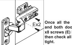
Once all the adjustments are complete and both doors are aligned, fix remaining x8 screws (E) into the other hinge plate holes then check all the other hinge screws are tight.
