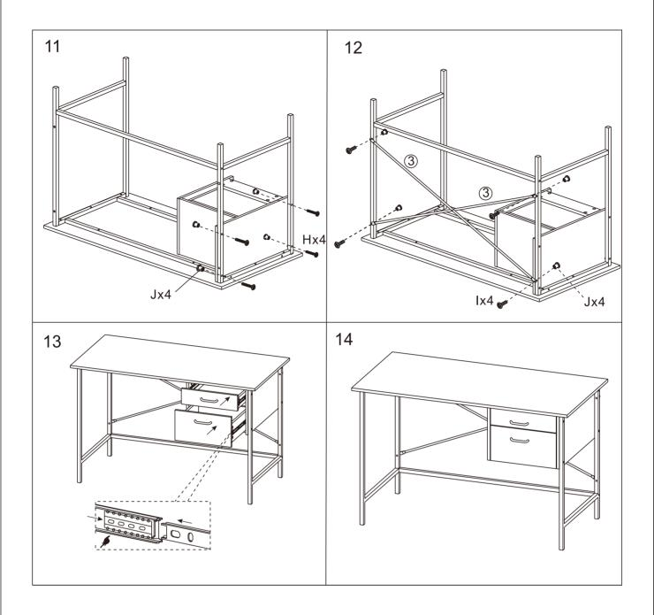
**Notes for installation:** Place **ALL** screws into the appropriate position and then tighten. **DO NOT** place and tighten one by one. If the desk comes with plastic caps, place over screws to cover holes.
