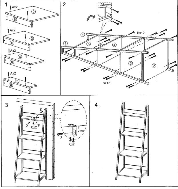
Notes for installation: Place ALL screws into the appropriate position and then tighten. DO NOT place and tighten one by one. If the shelf comes with plastic caps, place over screws to cover holes.
