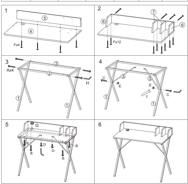
**Notes for installation:** Place **ALL** screws into the appropriate position and then tighten. **DO NOT** place and tighten one by one. If the desk comes with plastic caps, place over screws to cover holes.
