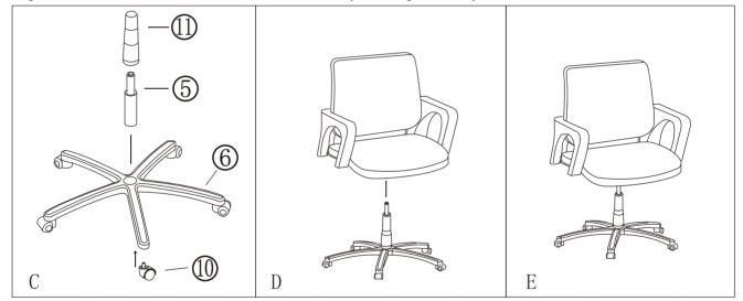
**Notes for installation:** Place **ALL** screws into the appropriate position and then tighten. **DO NOT** place and tighten one by one. If the chair comes with plastic caps, place over screws to cover holes.
