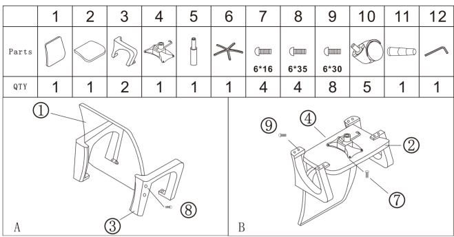
when inserting bolts 8 (step A) and bolts 9 (step B) we recommend that you leave these loosely tightened until all bolts have been inserted, only then tighten fully.
