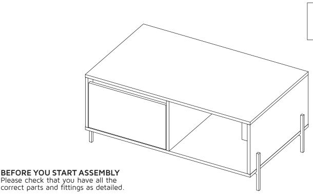
Height: 400 mm Width: 925 mm Depth: 550 mm
