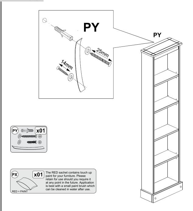
WARNING: CHECK FOR HIDDEN PIPES AND CABLES BEFORE DRILLING.
