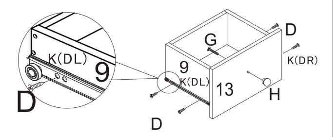
PLEASE ENSURE RUNNERS ARE FIXED TO THE CORRECT SIDES OF DRAWER. LEFT SIDE IS MARKED ON COMPONENT (DL) AND RIGHT SIDE IS MARKED (DR).
