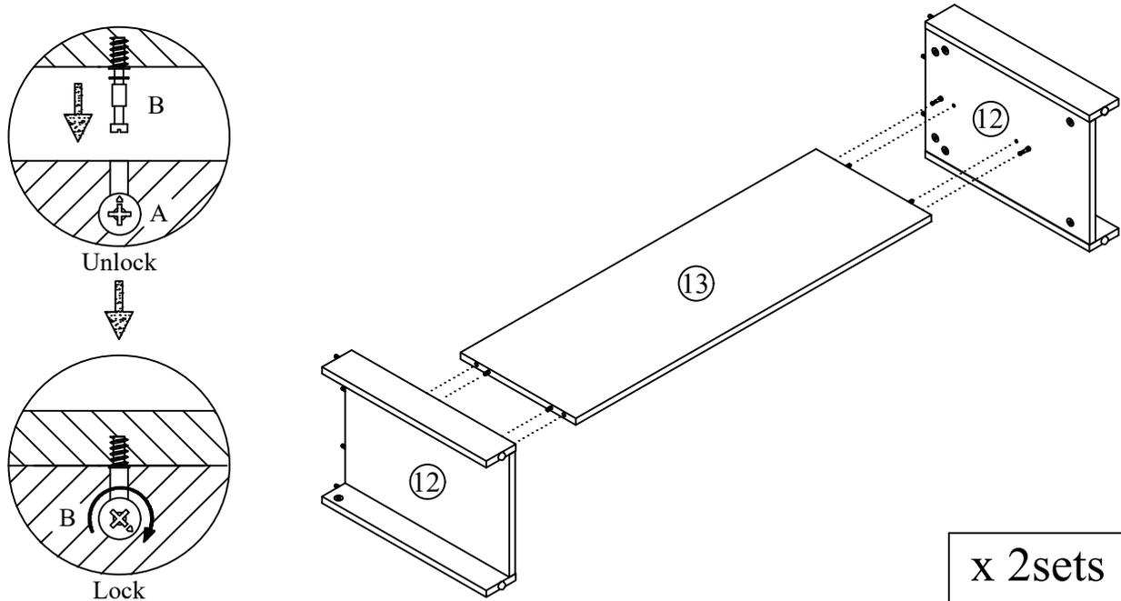
**9** Fix the bench side panels (12) and bench center panel (13) to the bench top panel (9) by using a screwdriver (not provided). **DO NOT** use any power tools as this may damage the frame and will invalidate any claim.
