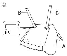
Step1: Put the screws in the holes, tight the screws, but not too tight, 90% is ok.
