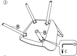
Step2: Put the screws in the holes, tight the screws, but not too tight, 90% is ok.
