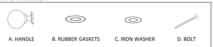
Step 1: Open the drawer, Unscrew Bolt(D), Take out Handles(A), Rubber gaskets(B) and Iron Washer(C), as below picture.
