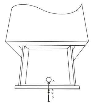
Step 2: Attach Handles(A)to the Drawer Front with Rubber gaskets(B), Iron Washer(C), and Bolt(D), as below picture.
