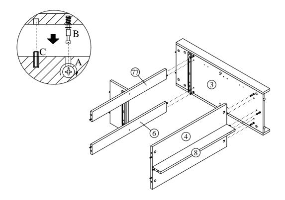
Attach the Front and Back Support Panel (6) & (7) to Left Panel (2) by screwdriver Vendor: S000398 (not provided).
