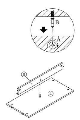
Attach the Front and Back Support Panel (6) & (7) to Right Panel (3) by screwdriver (not provided). Attach the Bottom Panel (4) and Plinth Panel (8) to Right Panel (3) by screwdriver (not provided). **DO NOT** use any power tools as this may damage the frame and will invalidate any claim.
