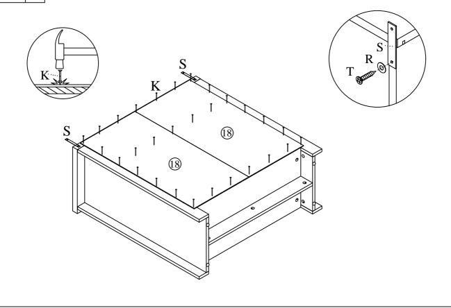
9 L 8 N 2 P 3 4 Q \ 2 Fix Hinges (O) onto Left and Right Panel (2) & (3) using screw (L) by screwdriver (not provided). Fix Metal Shelf Support (P) as shown
