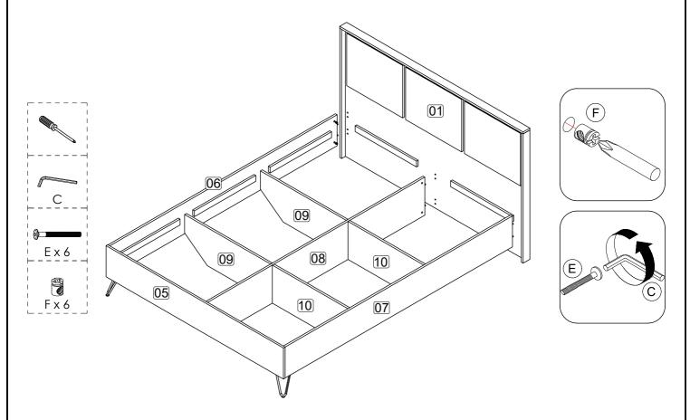
Step 8: Assemble bed board panel (11) between side rail (6), (7) and center panel (8).
