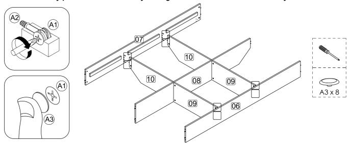
Step 4: Attach footboard panel (5) to side rail (6), (7) and center panel (8) using hardware A1 and A2 with a screwdriver (not provided).DO NOT use any power tools as this may damage the frame and will invalidate any claim.
