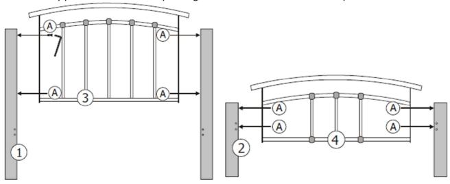
Step 2: Fix the side support (5) to the headposts (1) and footposts (2) using hardware part A. DO NOT use any power tools as this may damage the frame and will invalidate any claim.
