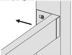
Step 5: Place hardware part D onto every end of each slat (7) then press firmly into the side supports (5). DO NOT use any power tools as this may damage the frame and will invalidate any claim.
