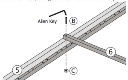
**Step 4**: Adjust both side supports (5) into the inner direction until the screws reach the end of the hole as shown. Tighten the screws for both side supports and the mid support.
