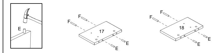
**Step 2:** Insert hardware part E using small mallet (not provided). **DO NOT use any power tools as this may damage the frame and will invalidate any claim.**
