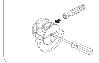
The head of the cam bolt goes into the open mouth of the cam nut. You then turn the cam nut so it tightens over the bolt.
