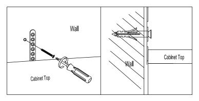
**NOTE:** Wall fixings are not supplied with this product as different wall materials require different types of fixing devices (such as Rawl plugs on brick work). You must use fixing devices suitable for the type of wall you intend to mount this product to. Please ensure that the head of any screw used has a diameter greater that the diameter of the mounting hole on the product and that the fixing is safe and secure before use.
