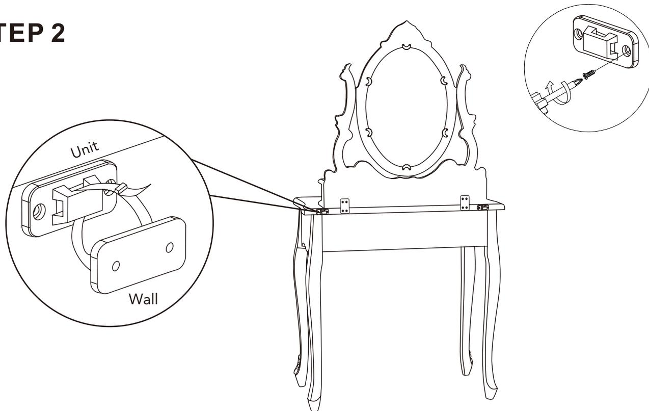
You will find two plastic brackets(B) pre fixed to the back of the unit. Then attach two plastic brackets(B) screwd into the wall as the image shows, use the plastic cable tie(C) connect each side plastic brackets(B).
