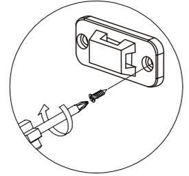
You will find two plastic brackets(A) pre fixed to the back of the unit. Then attach the two plastic brackets(A) screw into the wall as the image shows, use the plastic cable tie(B) connect each side plastic brackets(A).
