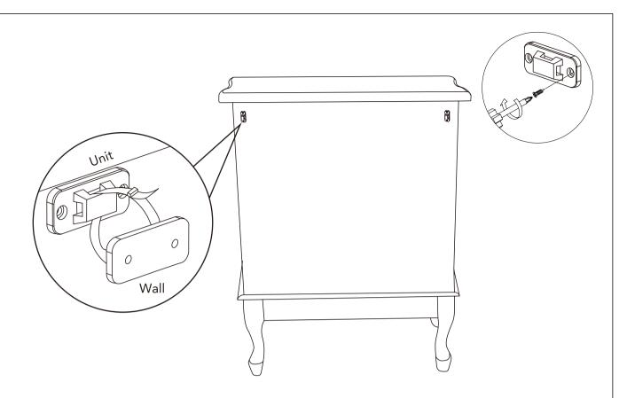
You will find two plastic brackets(A) pre fixed to the back of the unit. Then attach the two plastic brackets(A)
