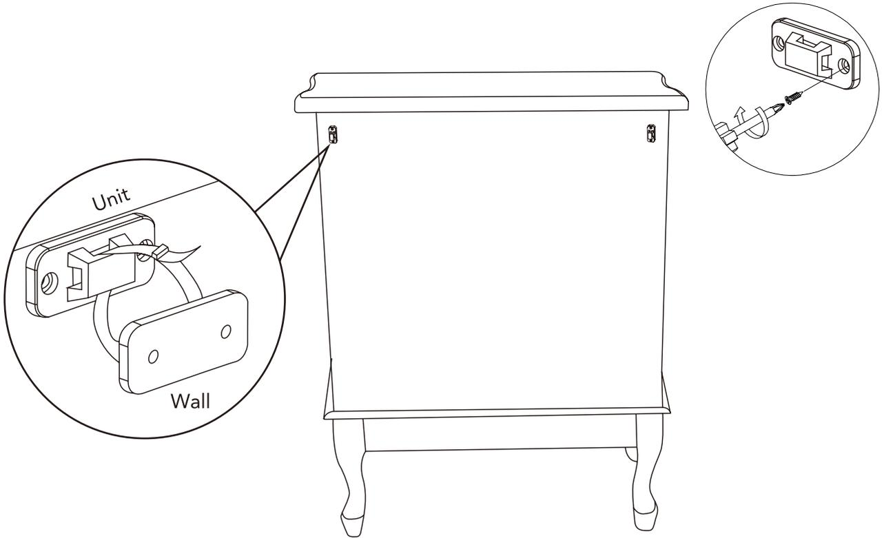
You will find two plastic brackets(A) pre fixed to the back of the unit. Then attach the two plastic brackets(A) screw into the wall as the image shows, use the plastic cable tie(B) connect each side plastic brackets(A).
