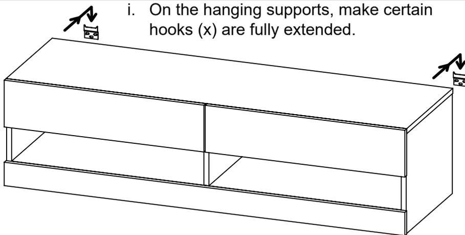
ii. With help, hang the cabinet onto the metal wall brackets by carefully aligning the end panels so they just miss the ends of the brackets. Turn upper screw(s) on either side until unit is horizontal.
