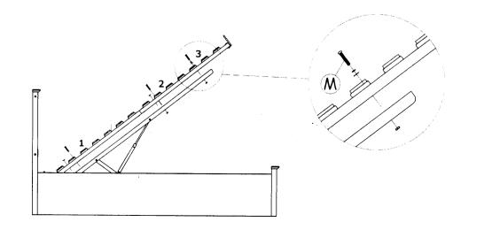
**Step 10**: Adjust the bed base making sure that the distance to the footboard is approximately 10 - 15 mm. Tighten all bolts and screws now.
