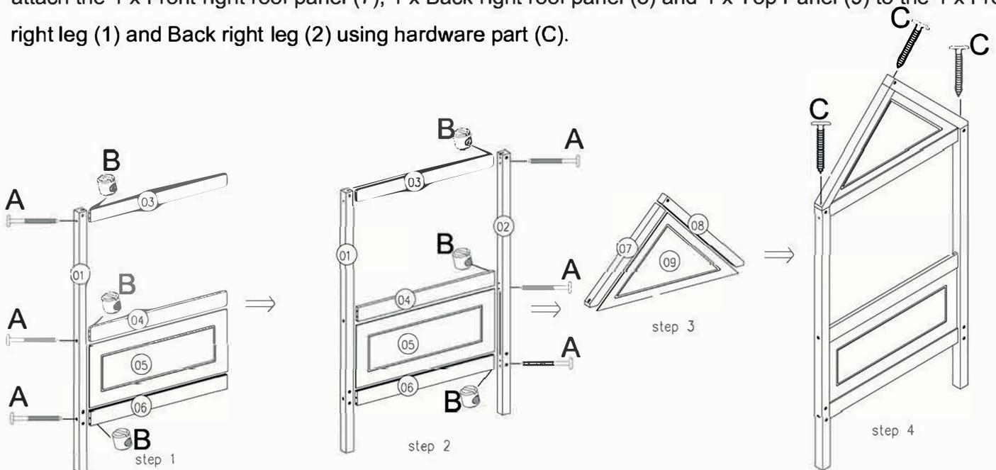
**Step 4:** Attach the 1 x Front left leg (22) and 1 x Back left leg (21) to the 1 x Top Head rail (3), 1 x Middle head rail (4), 1 x Bottom Panel (5) and 1 x Bottom head rail (6) using hardware parts (A) and (B). Then attach the 1 x Front left roof panel (17), 1 x Back left roof panel (18) and 1 x Top Panel (9) to the 1 x Front left leg (22) and Back left leg (21) using hardware part (C).
