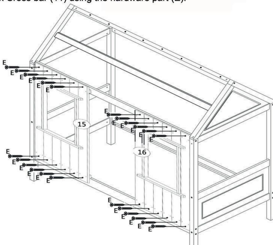
Attach 1 x left bed roof (14) and 1 x right bed roof (19) using the dowels. Once attached apply remaining roof panels ensuring they are aligned using hardware part (E).
