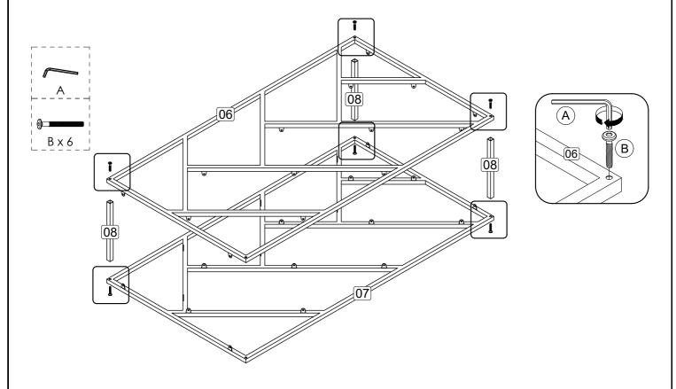
Step 2: Attach Top panel (1) to Metal Front (6) and Metal Back (7) using hardware C with a screwdriver (not provided).DO NOT use any power tools as this may damage the frame and will invalidate any claim.
