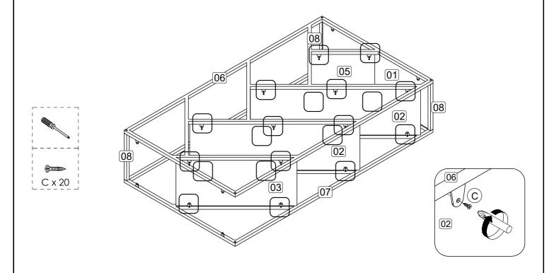
Step 4: Attach Shelf panel (4) to Metal Front (6) and Metal Back (7) using hardware C with a screwdriver (not provided).
