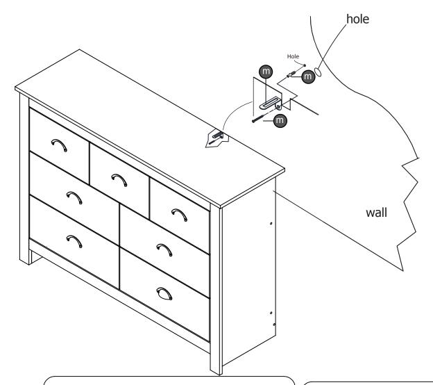
NOTE: The wall fixing plug supplied with this product is suitable for solid and brick walls.
