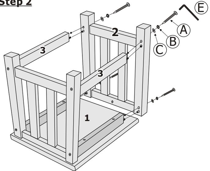
Then, attach another Side Frame (2) to the Chair Seat (1) and Stretcher (3) using screw (A), spring washer (B) and flat washer (C).
