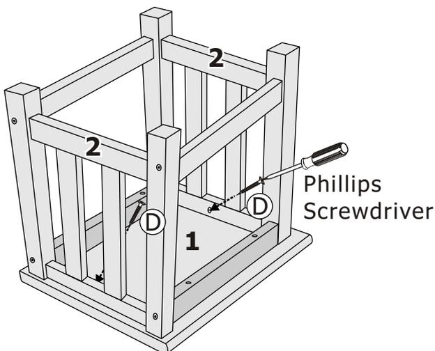
Attach the Side Frame (2) to the Chair Seat (1) using screw (D). Use a Phillips Screwdriver (not provided) to drive screw (D).
