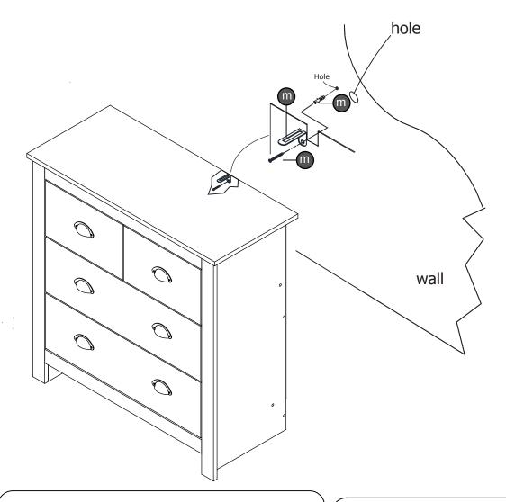
NOTE: The wall fixing plug supplied with this product is suitable for solid and brick walls.
