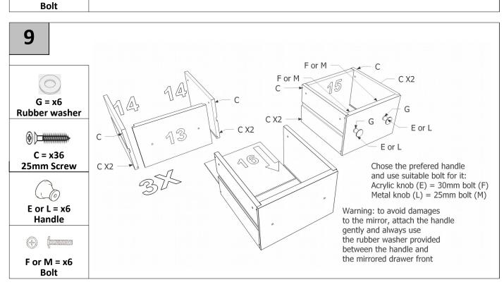
gently and always use the rubber washer provided between the handle and the mirrored drawer front
